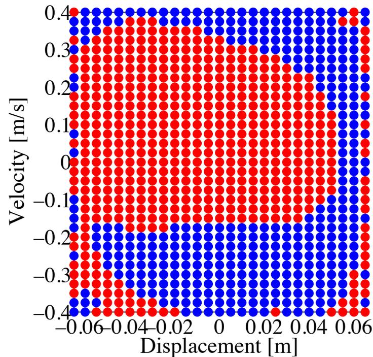
**Even if the system is responding in the high-energy solution, it can easily drop down to the low-energy solution when subjected to disturbances.**
